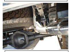
**6.** Install the exit pipe Item # B onto the over axle pipe. Do not tighten. Keep everything loose until you have proper clearance.
