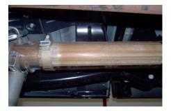
2. Install Item # A on to your factory exhaust using clamp # D to secure. Do not tighten.
